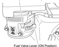
Figure 16 - Fuel Valve Lever On, Choke Lever Closed (Model PGH7500IE Shown)
